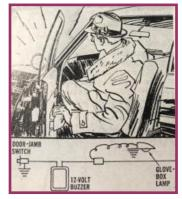
NO FLAT (DEAD) BATTERIES A headlight reminder could save you a dead battery. Put in an additional door-jamb switch on the driver's side, connect it to a 12 volt or 6 volt (whichever flavor your car may be) buzzer and in turn to the glovebox lamp (only hot when headlights are on). Open the door the buzzer sounds.
