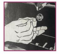
**BROKEN KEY** When a key breaks off in a door, trunk, or ignition lock and you cannot get the broken piece out, grind down a section of saw blade so it fits next to the broken piece in the lock. Pull back gently, the blade teeth will pull out the broken piece.
