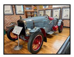
There were many unique cars each one having its own story. This cut-down '22 Ford Model T roadster body, was mounted on an altered '31 Ford Model A frame, and powered by a highly modified Cadillac V-8. Built in 1955 by Norm Grabowski, the car appeared on the popular TV show, "77 Sunset Strip." Driving the car in the series was "Kookie" Kookson, played by actor and teen-age heart throb, Edd Byrnes.
