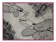
**STOP LEAK** When there is consistent leakage from a coupling on a copper fuel line, here is a fix. Loosen the coupling and bend a ring of bare copper wire around the tubing just behind the flared end. Draw up the coupling and the ring will seal the union. If necessary, use two windings of wire.
