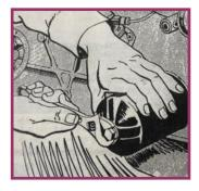
**BETTER SEAL** When installing an oil filter element in a top cover or shell type casing, be sure to hold the cover or shell tightly in place while tightening the center bolt. If you keep the shell from turning, the gasket will seal and assure freedom from leaks.
